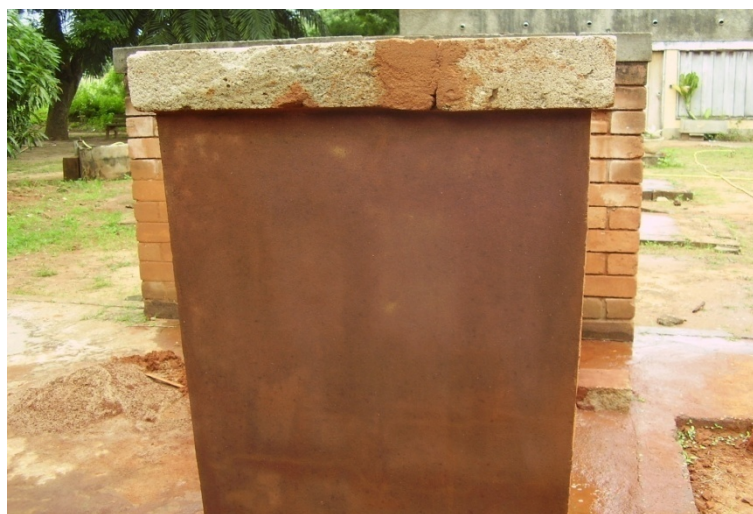
Fig. 5 Clay, sand, cement and locust bean fruit husk's extract.
